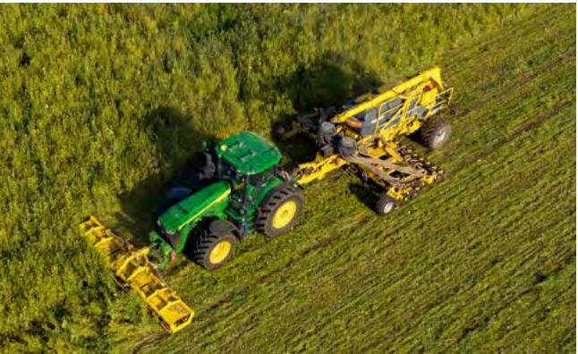
Aggregation with no-till seed drill DIRECTO NO
