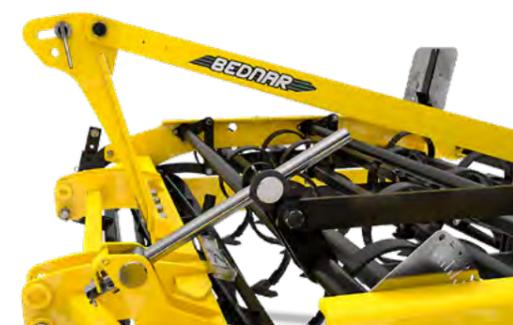
The working depth is set using a trapeze thread with a removable handle. Precise setting along the entire working span is ensured with a numerical order and an indicator individually for each section.
