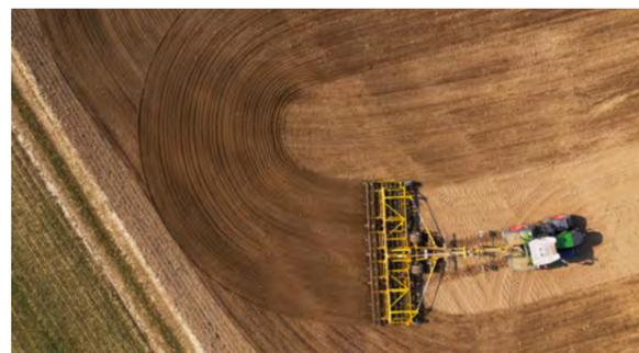
The design of the SWIFTER SE cultivator enables turning the machine at headlands without having to lift the working sections. We recommend turning at headlands at lower working speed and a higher turning radius. The telescopic connecting rods stabilize the side frames not only when turning, but also at higher working speed.
