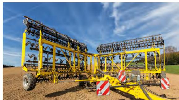
The SWIFTER SE wide cultivator can be easily folded into transport position from the tractor cabin. The fully hydraulic folding of the working sections forward to the drawbar provides compact transport dimensions of up to 3 metres of transport width, required for transport on roads in EU countries.
