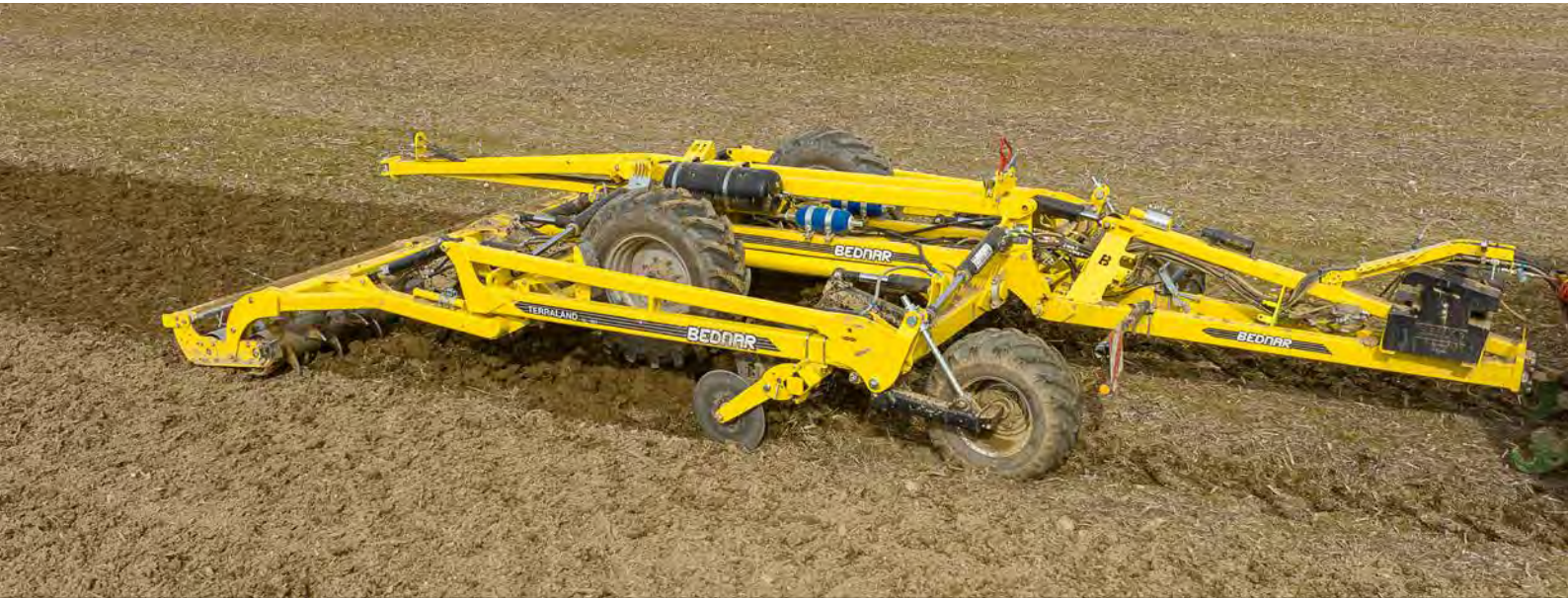
TERRALAND is a chisel plough designed for deep soil cultivation, soil profile aeration and disruption of the hardened soil layers to a depth of 65 centimetres.
