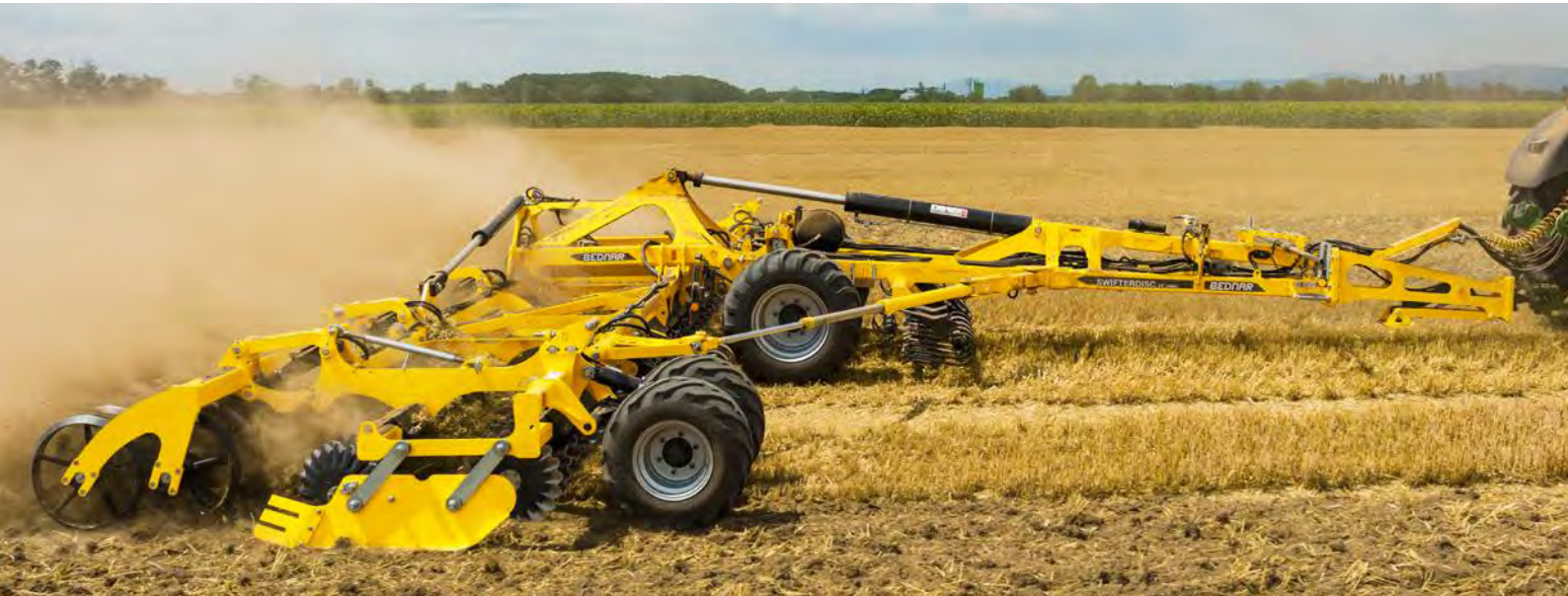
SWIFTERDISC is a highly versatile, short disc cultivator, suitable for quality and fast stubble cultivation up to the depth of 14 centimetres, as well as for seedbed preparation.
