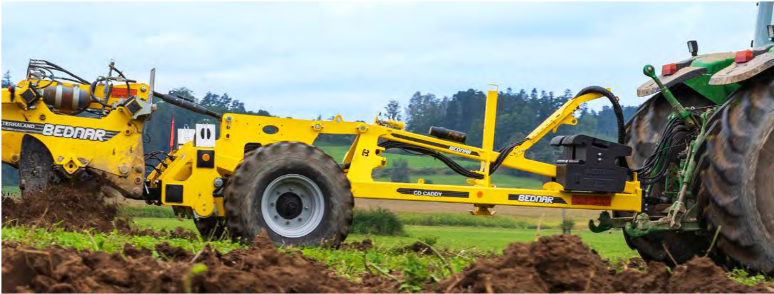
CADDY CD is a versatile tool carrier to be aggregated with tractors without the three-point hitch. The GALAXY GE trailed packers are used for quality clod crumbling and back soil profile closure.
