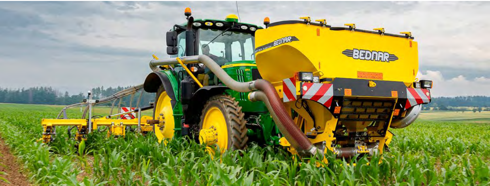
FERTI-BOX and SEED BOX SB are model series of mounted hoppers for fertiliser or seed application with a capacity from 1,600 to 3,000 litres.
