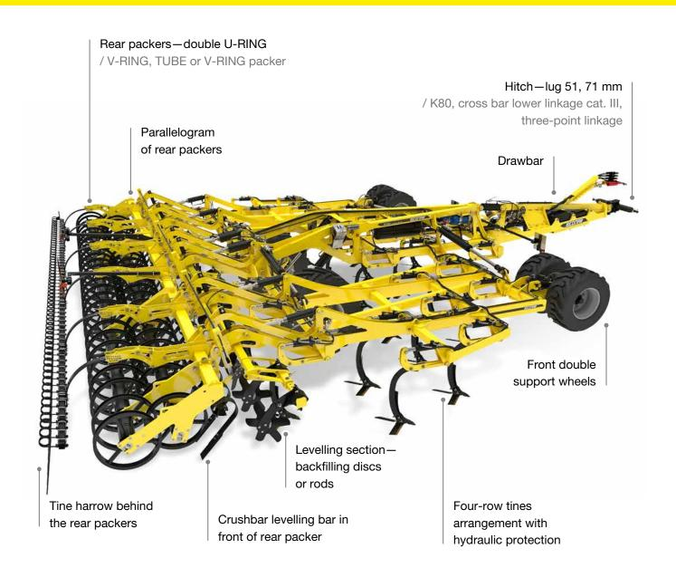
The FENIX FO\_PROFI deep cultivator is a new generation of cultivators for intense shallow soil cultivation after harvest, as well as in-depth cultivation of up to 35 centimetres prior to crop establishment. The FENIX FO\_PROFI semi-mounted cultivator has tines arranged into four rows in the shape of an arrow. The well-thought-out design reduces draft resistance and tractor output demands.
