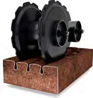
Double Presspack Packer The PRESSPACK is a heavy steel packer that consists of two rows of steel rings. This type of packer is suitable for heavy soils. It offers a great crumbling and compacting effect.
