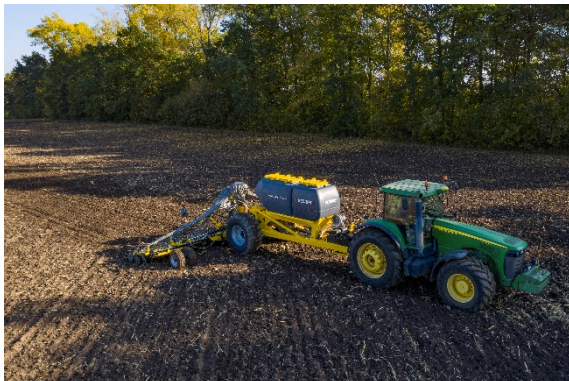
Three-point hitch, category IV, for easy aggregation of the COMBO SYSTEM CS pressurized hopper with other BEDNAR machines
