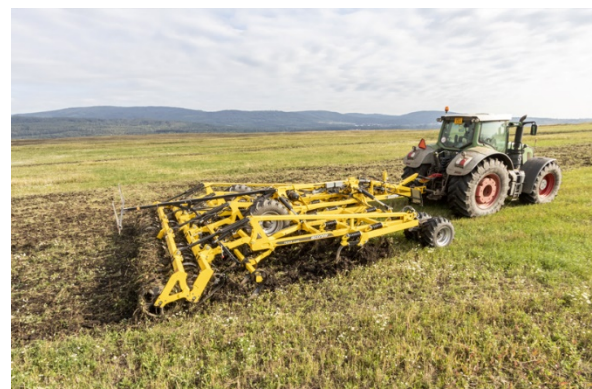
3 or 4 rows of shares with constant geometry easily work even in extreme conditions
