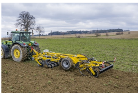
ACTROS RO has optional rear packers according to the type of soil conditions
