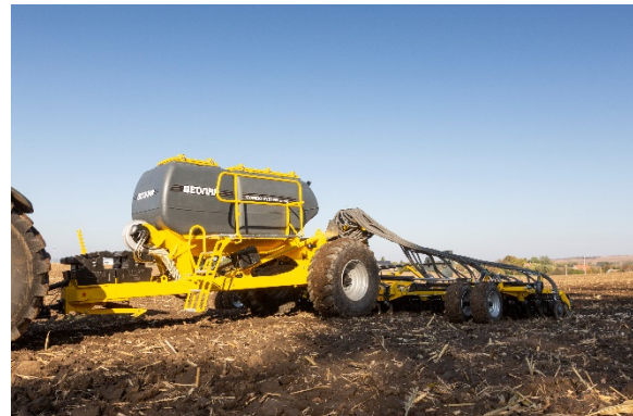
Double-chamber pressurized hopper aggregated with the CORSA CN seeding bar
