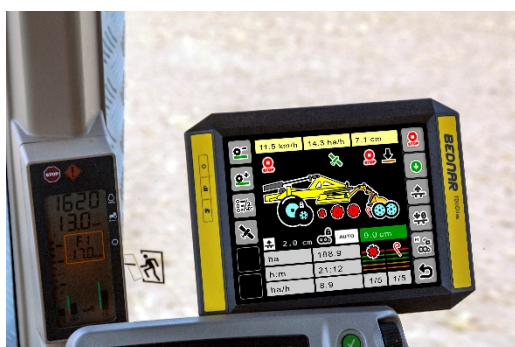
The EH-Set electrohydraulic machine control via the ISOBUS standard
