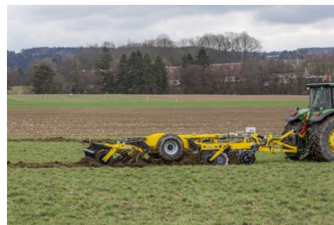
The combined cultivator with two rows of discs, 660 x 6 mm, and two rows of shares with massive spring protection
