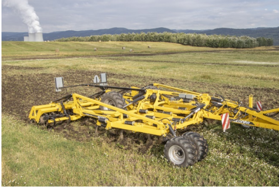
The integrated axle provides for fast turning at headland
