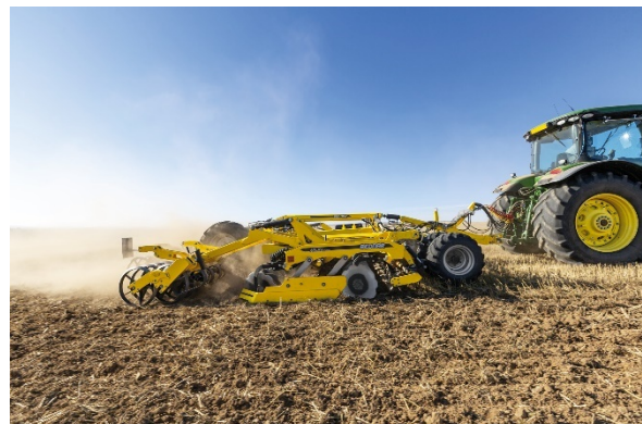
The new Bednar machine, ATLAS AO_PROFI performs stubble cultivation at 16 cm in a stubble field
