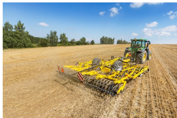
The universal cultivator is doing intense stubble cultivation at up to 15 cm – absolutely straight bottom of the soil profile
