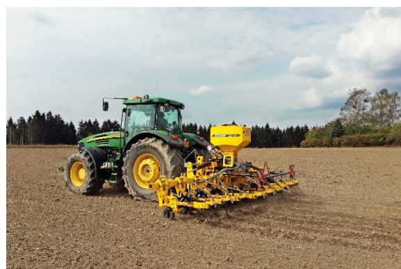
The ROW-MASTER RN cultivator equipped with ALFA DRILL is establishing catch crop
