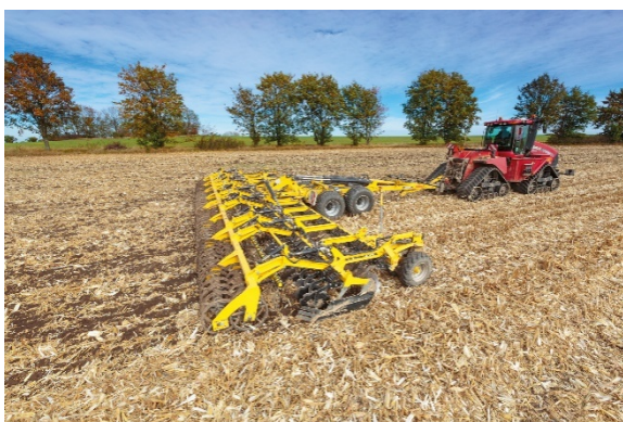
The wide ATLAS AE_PROFI disc cultivator easily processes a large quantity of crop residue
