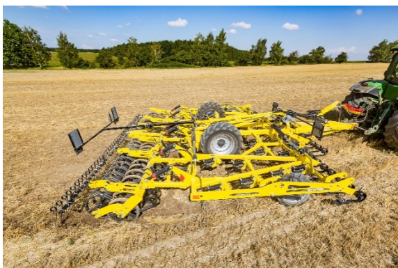
VERSATILL VO_PROFI allows working without rear packers
