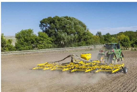
ALFA DRILL in combination with the STRIEGEL-PRO PE straw harrow manages to seed cover crop or grasses
