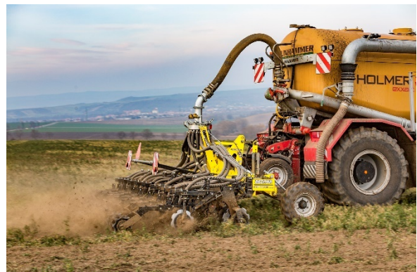
The novelty in the BEDNAR portfolio has individual row unit mounted on a parallelogram
