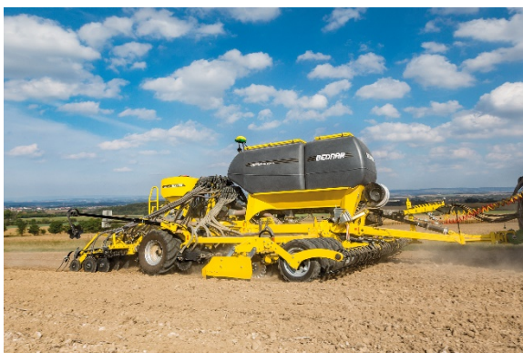
The new OMEGA OO_FL seed drill provides the option to place fertiliser in the inter-row between the seeds, or together with the seed
