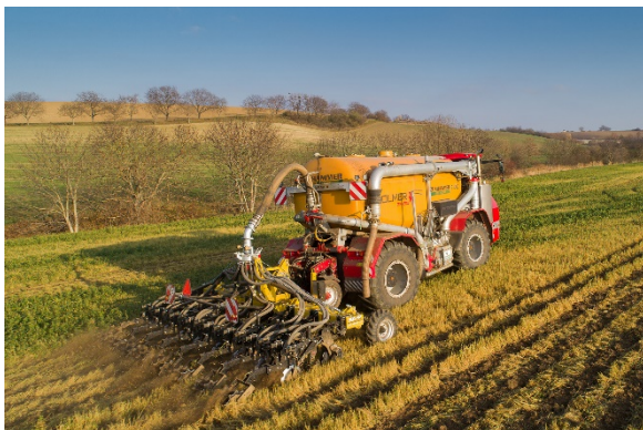
STRIP MASTER EN disturbs the compacted layers and places fertiliser at two layers
