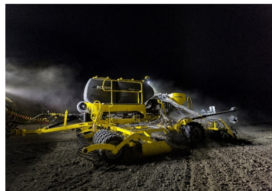
Precise seed placement at an identical depth along the entire width of the machine thanks to the PSP system
