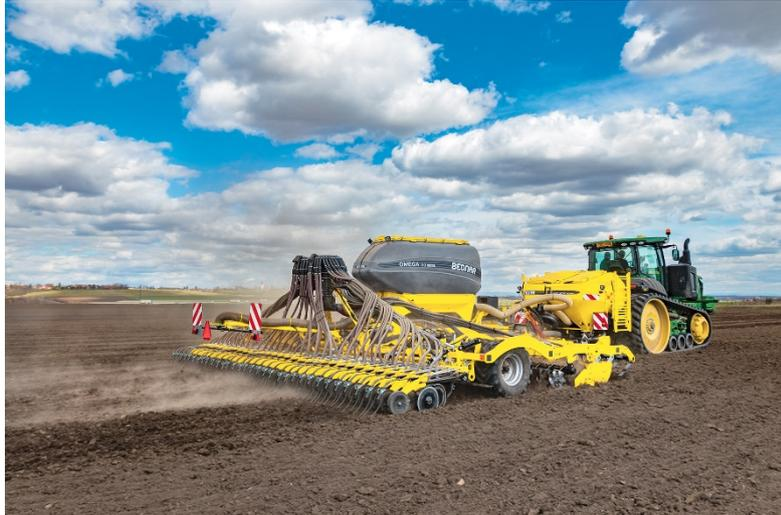
*The OMEGA OO 8000 L seed drill in aggregation with FERTI-BOX FB, a fertiliser hopper*
