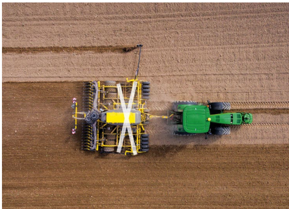
The OMEGA OO_L seed drill has "X"-shaped disc sections, ensuring precise tracking of the tractor by the seed drill.
