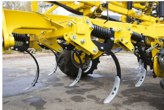
Shares with NON-STOP protection for seedbed preparation and stubble cultivation up to 15cm in heavier conditions
