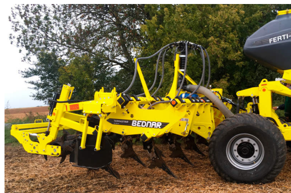
TerraStrip in combination with Ferti-Cart FC 3500 designed for profile fertilization
