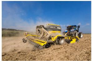
Machines from the OMEGA series allow various types of crops to be seeded with an inter-row spacing of 12.5 or 16.5cm, with a highly variable seed rate both in the conventional and minimization soil tillage system. The PSP system comes as standard – the disc seed coulters place seeds at an identical seed depth along the entire width of the machine and impeccably contour unevenness of the ground both in the longitudinal and transverse direction.
