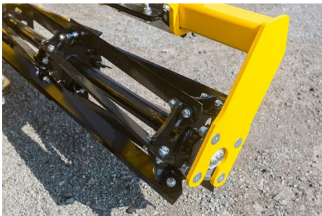
Trash Cutter is designed for SWIFTERDISC disc cultivators and STRIEGEL-PRO straw harrow
