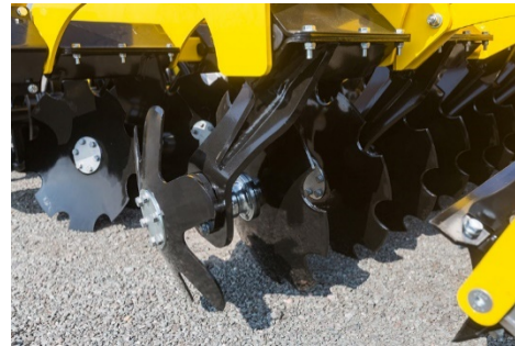
The screw joints between discs, bearing boxes and tines are protected against undesirable loosening with anti-vibration washers
