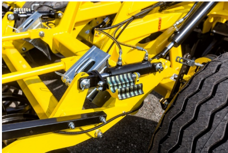
A fast setting of working depth using spacing washers on hydraulic cylinders
