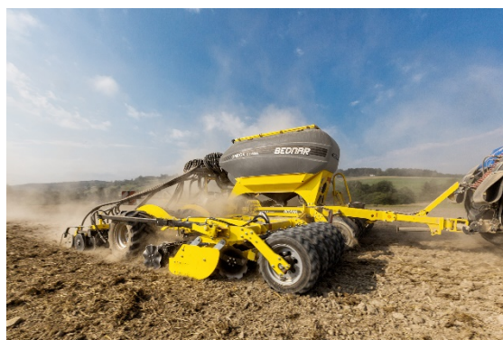
The OMEGA OO_L seed drills are equipped with discs with a diameter of 460 mm
