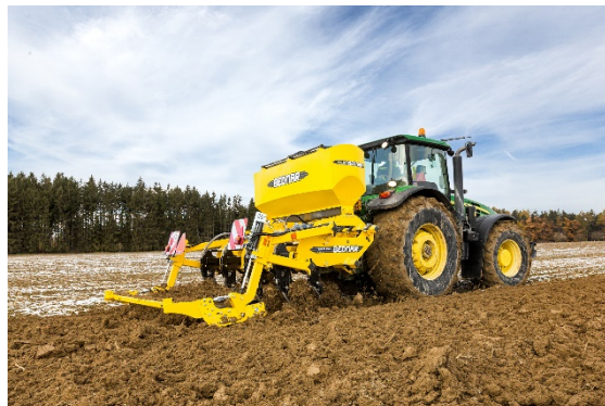
FERTI-BOX FB 1500 TN with the capacity of 1500L can be mounted on the new as well as the current TERRALAND chisel ploughs
