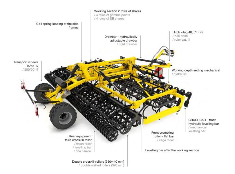
The semi-mounted SWIFTER SO\_PROFI models are available with a working width of 5 and 6 metres.
