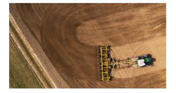
The design of the SWIFTER SE cultivator enables turning the machine at headlands without having to lift the working sections. We recommend turning at headlands at lower working speed and a higher turning radius. The telescopic connecting rods stabilize the side frames not only when turning, but also at higher working speed.
