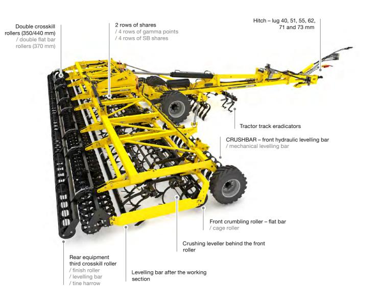
The SWIFTER SE model line offers seedbed cultivators with a working width from 8 to 12 metres. The high working speed allows achieving high daily outputs with these machines. An advantage of SWIFTER SE is the independent suspension of the working sections for perfect terrain tracing.
