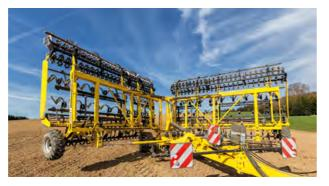
The SWIFTER SE wide cultivator can be easily folded into transport position from the tractor cabin. The fully hydraulic folding of the working sections forward to the drawbar provides compact transport dimensions of up to 3 metres of transport width, required for transport on roads in EU countries.
