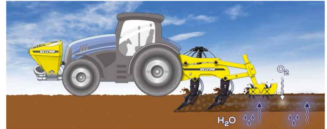
SPRING – SPRING PRE-SOWING PREPARATION USING A SWIFTER WITH SB SHARES
