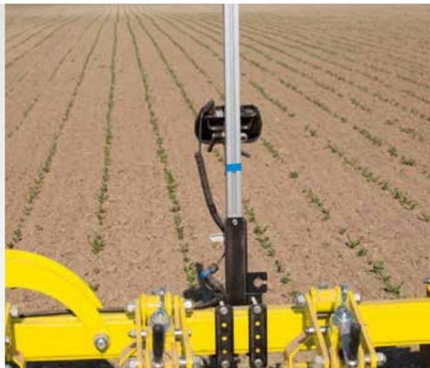
The height and angle of the camera can be set based on the current stage of the crop growth.
