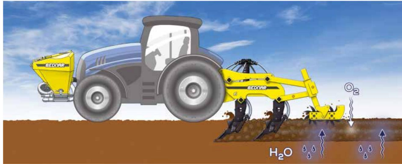
SPRING – SPRING PRE-SOWING PREPARATION USING A SWIFTER WITH GAMMA TINES
