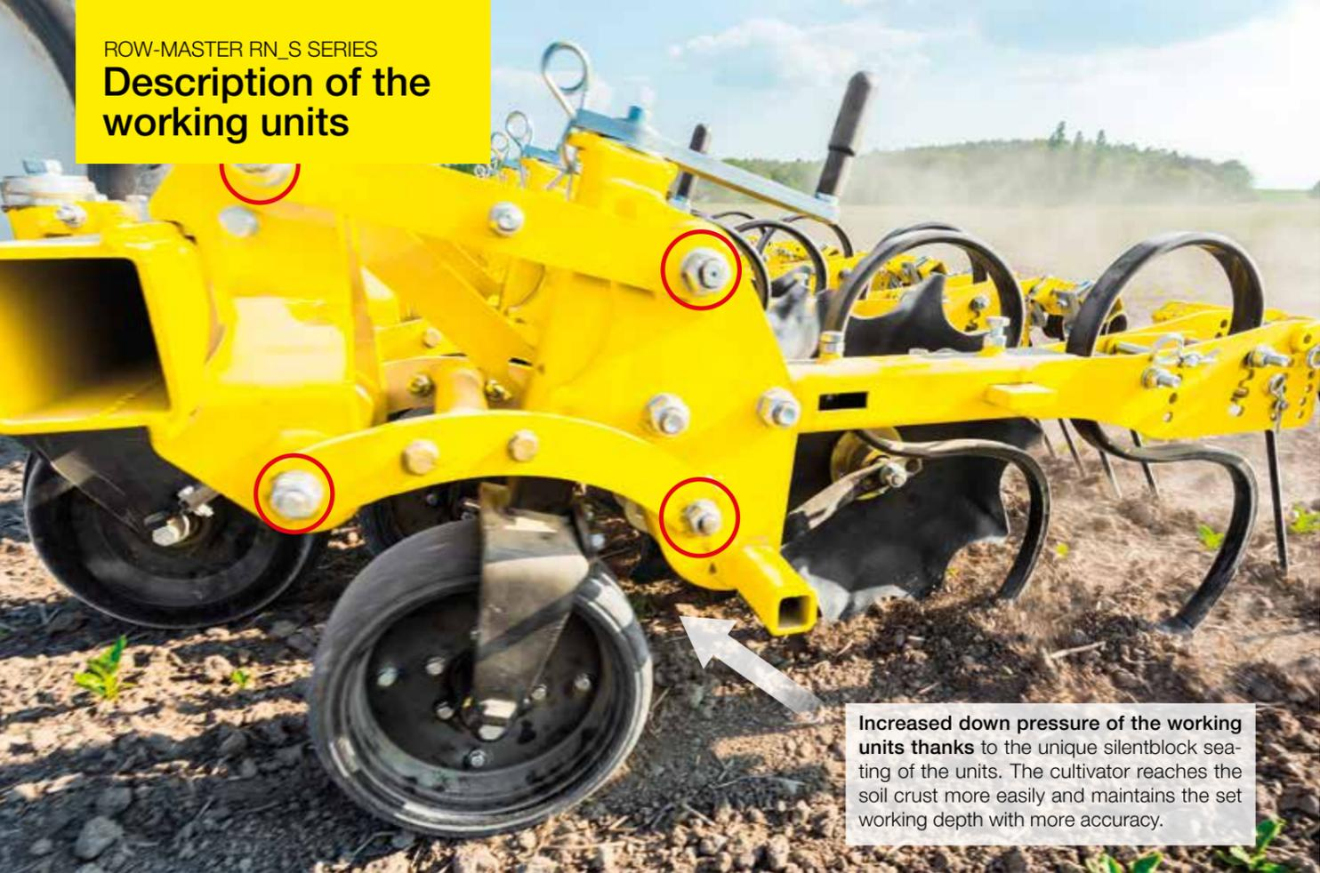
Increased down pressure of the working units thanks to the unique silentblock seating of the units. The cultivator reaches the soil crust more easily and maintains the set working depth with more accuracy.
