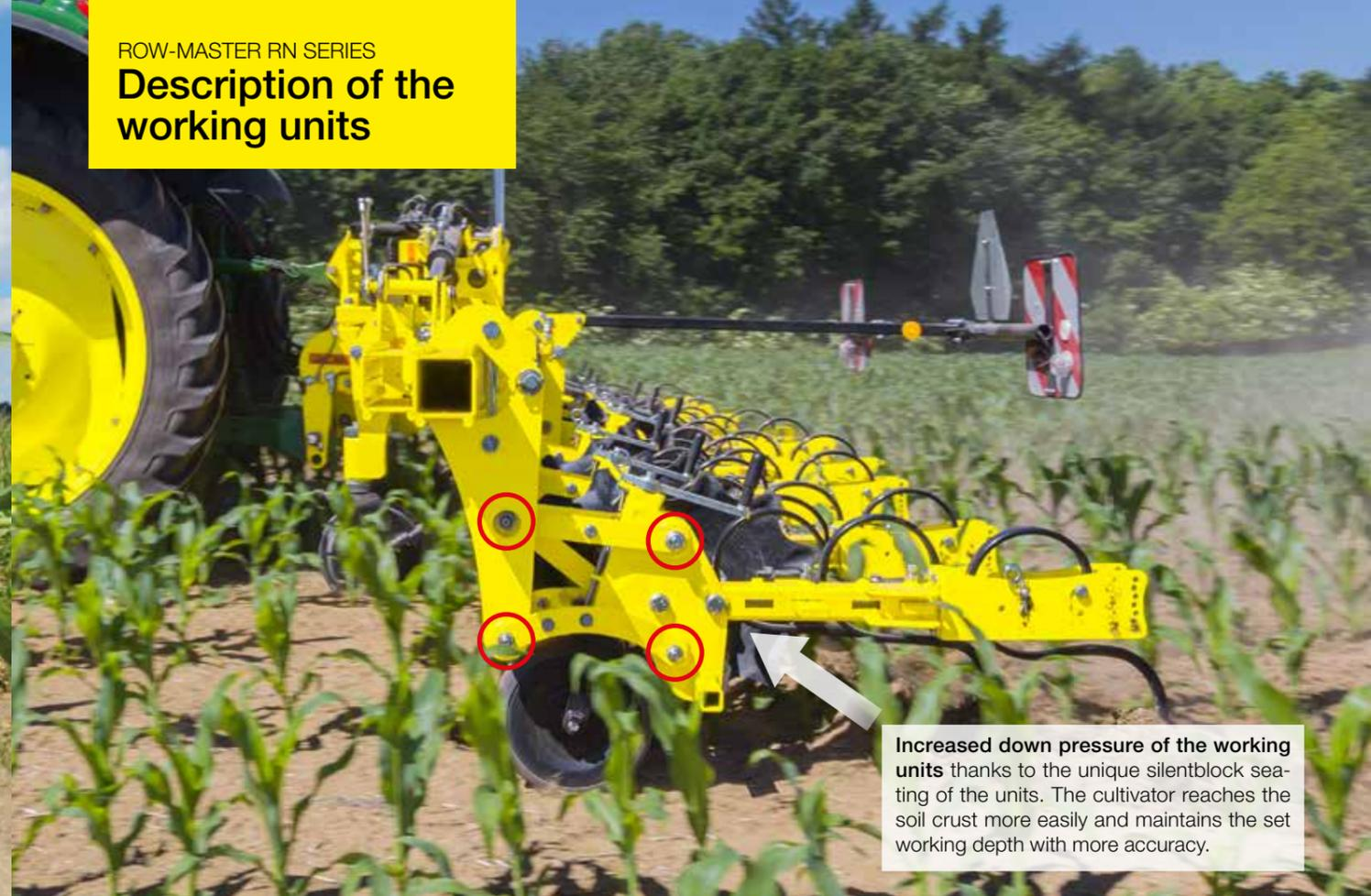
**Increased down pressure of the working units** thanks to the unique silentblock seating of the units. The cultivator reaches the soil crust more easily and maintains the set working depth with more accuracy.
