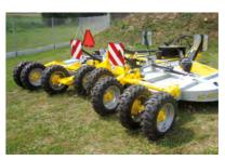
The MM 7000 rotary cutter comes as a standard 8 wheel model. The MZ rotary cutter comes in a standard 6 wheel model but can also be customised to come in an 8 wheel version. The wheels can be filled with foam to prevent puncture.
