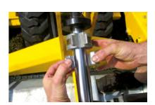
The mulching height of the MZ and the MM machine is set centrally with the help of hydro clips on the hydraulic cylinder conduit of the machine's central axle. Adjustment of the setting is done swiftly and with ease.
