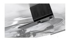
To increase the crumbling effect of the front parts of the mulching zone, they have been equipped with counter blades that complete the cutting of the mulched material. The quality of the mulched material is therefore increased.
