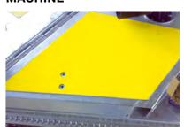
BEDNAR rotary cutters can be equipped with plates that cover the main frames. These plates are smooth and minimise sticking of the vegetal residue to the machine.
