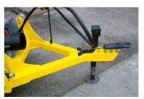
The MZ and MM rotary cutters are hooked up to the upper or lower tractor tow with a ring that has a diameter of 40, or 50mm in size leading on to a K80 tow.
