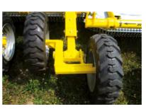
A central swinging axle helps to overcome uneven surfaces whilst maintaining working height. Thanks to the axle the machine is able to operate smoothly even on extremely rough fields and pastures.
