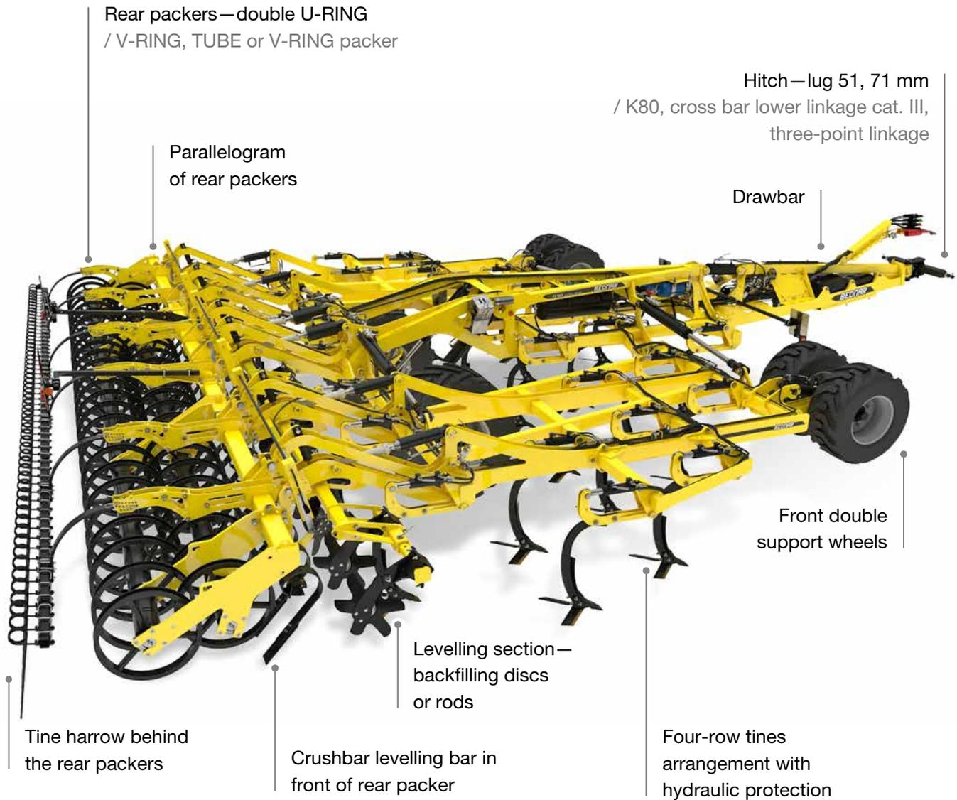
**The FENIX FO\_PROFI deep cultivator** is a new generation of cultivators for intense shallow soil cultivation after harvest, as well as in-depth cultivation of up to 35 centimetres prior to crop establishment. The FENIX FO\_PROFI semi-mounted cultivator has tines arranged into four rows in the shape of an arrow. The well-thought-out design reduces draft resistance and tractor output demands.
