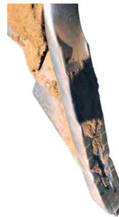
Long-Life chisel after processing 700 ha of soil
